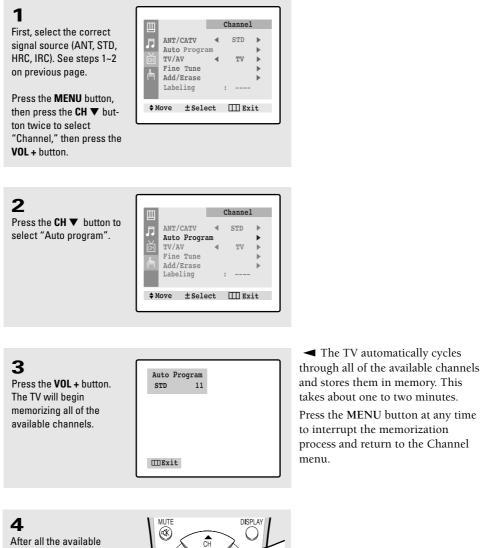
takes about one to two minutes. Press the MENU button at any time to interrupt the memorization
